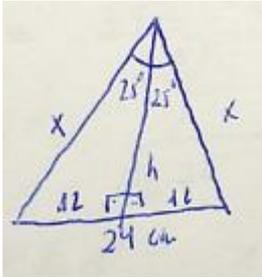
$$\begin{aligned} \text{sen } 25^\circ &= \frac{12}{x} \Rightarrow x = \frac{12}{\text{sen } 25^\circ} \Rightarrow \boxed{x = 28,39 \text{ cm}} \\ &\text{Cada lado} \\ \text{tg } 25^\circ &= \frac{12}{h} \Rightarrow h = \frac{12}{\text{tg } 25^\circ} \Rightarrow \boxed{h = 25,736 \text{ cm}} \\ \text{Área} &= \frac{24 \cdot 25,73}{2} \Rightarrow \boxed{\text{Área} = 308,76 \text{ cm}^2} \end{aligned}$$
